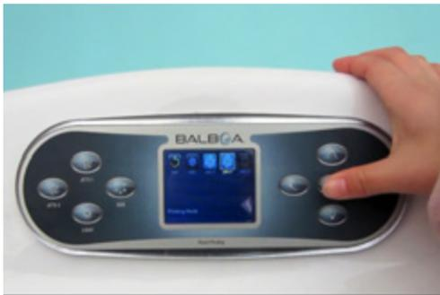
Now the hot tub is full of water, replace the filters and turn on the hot tub from the isolator.
